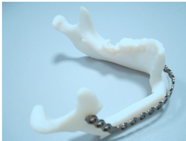
Figure 11 Customized Titanium plate and reconstruction mandible RP model
