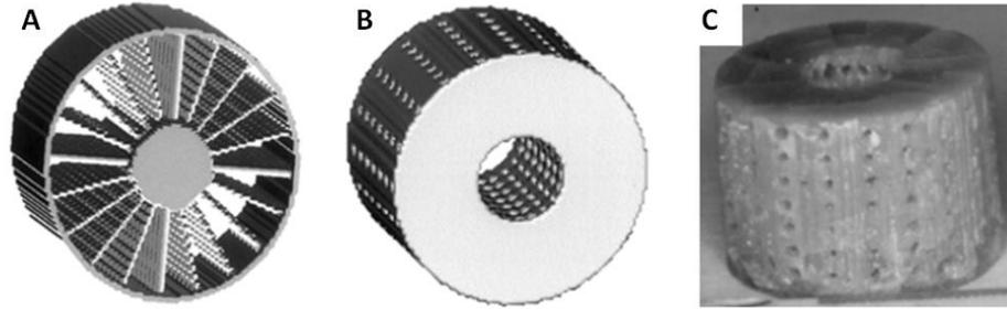
**Figure 2.** Indirect scaffold fabrication; a) a mold “negative” created via SLA; b) CAD representation of the desired scaffold architecture; c) the final scaffold composed of sintered HA [40]
