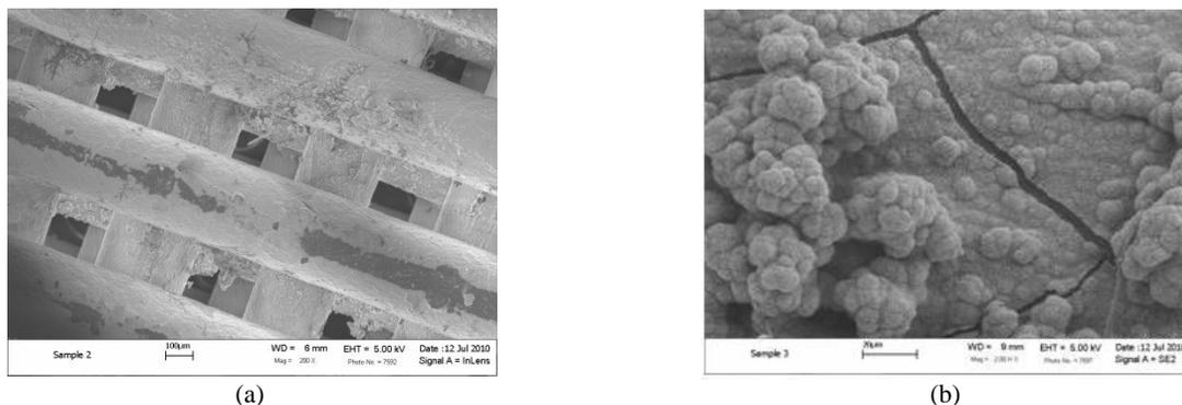
**Figure 8.** a) Mineralization of the top and second layer of an ABS scaffold (200x zoom). b) Clusters of minerals and small cracks formed on the mineral coating (2000x zoom)
