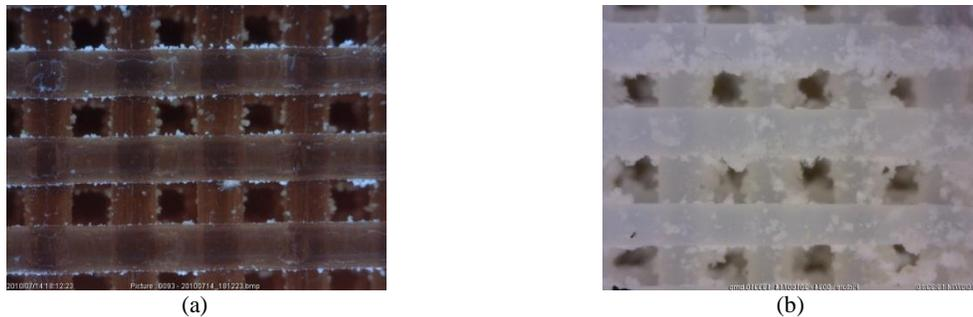
**Figure 7.** a) ICW pattern has slight mineral deposits following NaOH etch, but is not heavily coated (b) like the ABS pattern following plasma-etch.
