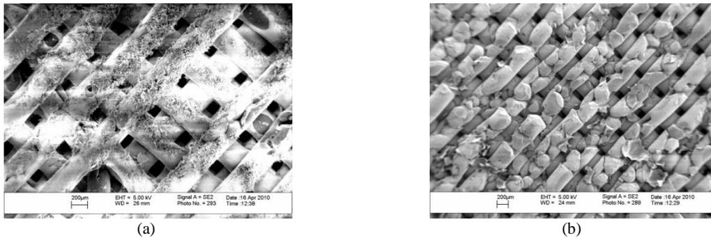
**Figure 4.** a) FESEM of an untreated ABS scaffold mineralized with SBF 5x (100x zoom); b) FESEM of the bottom of the same scaffold (70x zoom).
