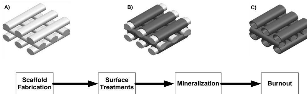
**Figure 3.** Proposed scaffold fabrication process; a) scaffold pattern is fabricated via FDM, b) scaffold pattern after surface treatment and ceramic mineralization, c) biocompatible scaffold with micro-tubes formed by removing the pattern material.
