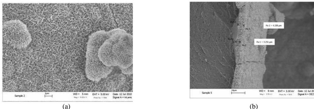
**Figure 9.** a) The mineral coating and clusters have the same surface morphology (10000x zoom). b) The mineral coating is ~0.003-0.004 mm thick (3.78k x zoom).
