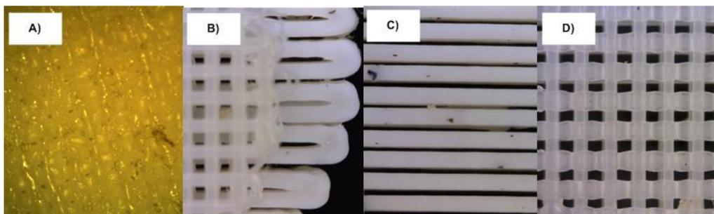
**Figure 5.** A) Scaffolds not printed on a base had fused bottoms and sometimes failed during printing. B) Scaffold pattern printed on a support material base. C) The scaffold pattern removed easily from the base. D) Scaffolds printed on a base did not have a fused base and had consistent pore sizes throughout.
