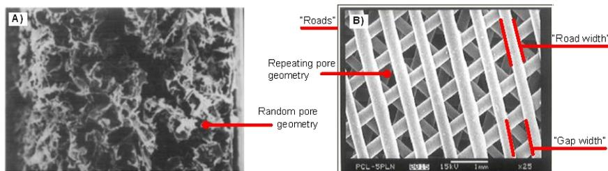
**Figure 1.** Scaffolds fabricated via (a) traditional stochastic (a PLLA “foam” created by a solvent casting particulate-leaching technique [16]) and (b) additive manufacturing (a PCL scaffold fabricated via FDM [7]) techniques
