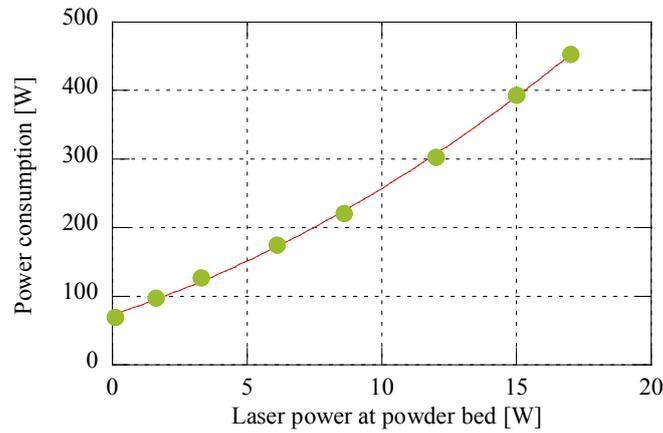
**Figure 12** Relationship between energy consumption and laser irradiation at powder bed
