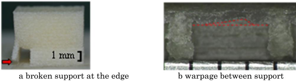
**Figure 6** Failure of support
