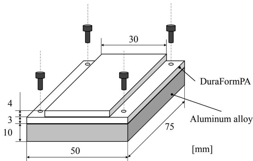
Figure 2 Base plate structure
