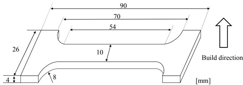
**Figure 4** Tensile test piece
