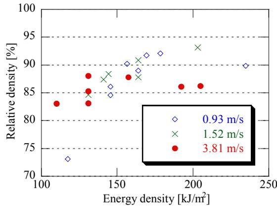
**Figure 5** Relationship between relative density and energy irradiation per unit area
