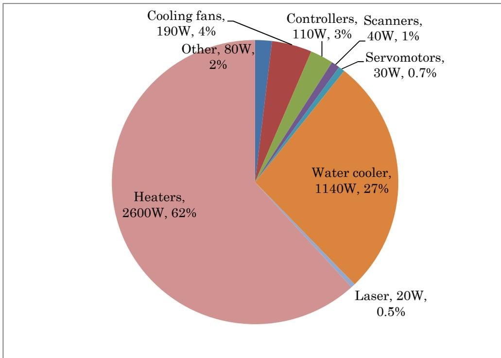
**Figure 1** Power consumption of a laser sintering machine in idling state after warm up is finished.
