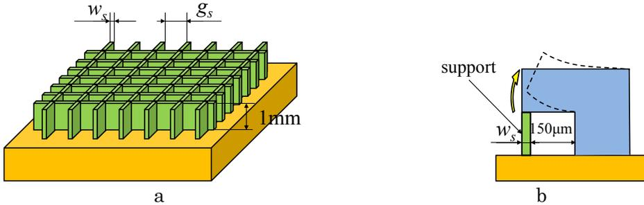
**Figure 3** Mesh type support structure and its parameter optimization
