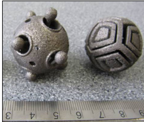
Figure 7 Anchorless Bi3Zn eutectic parts fabricated using ASLM
