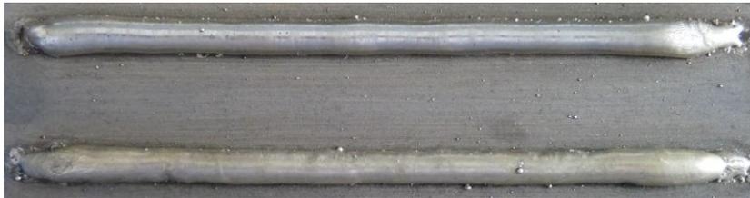
**Fig. 14:** Comparison of two-layer systems: a) first dragging, then pushing (top) b) first pushing, then dragging (bottom)
