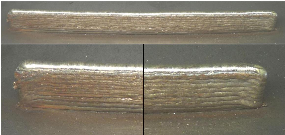
**Fig. 15:** Bi-directional welded structure with fixed height offset with a size of 260 x 26 x 6 mm (top) Ends of the structure without build-up or lack of material (bottom)
