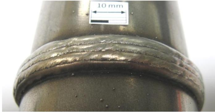
**Fig. 7:** Seam helix with even surface
