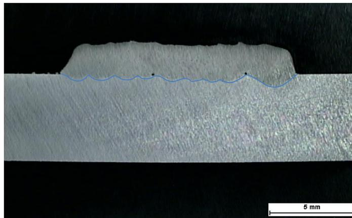
**Fig. 5:** Low dilution and even surface with material combination A
