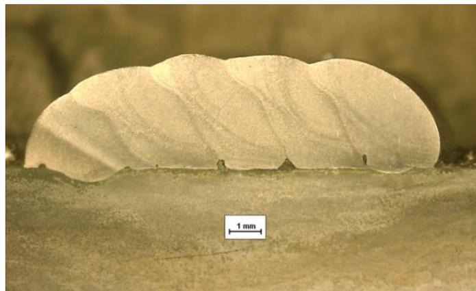
**Fig. 6:** *Cross section of material combination B*
