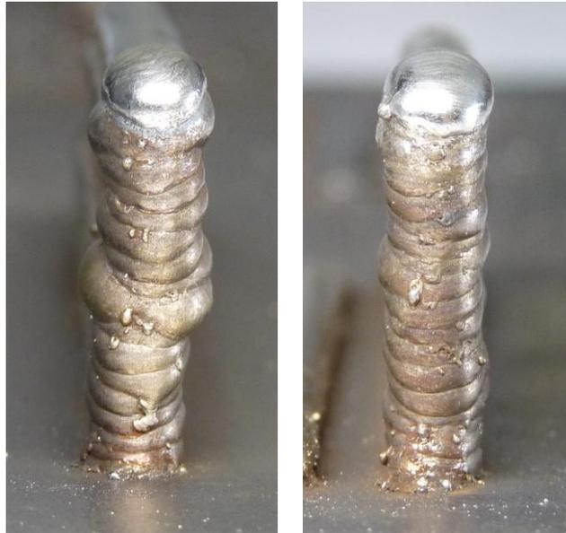
**Fig. 10:** Comparison of structures built with laser stabilization (right) and without (left)
