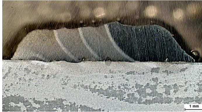
**Fig. 4:** Low dilution of base and deposition material
