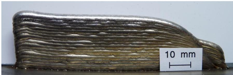
**Fig. 12:** Deposit build-up at beginning and lack of material at end of structure
