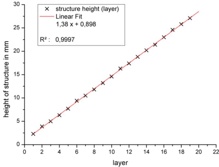
**Fig. 11:** Linear progression of the structural height with each layer
