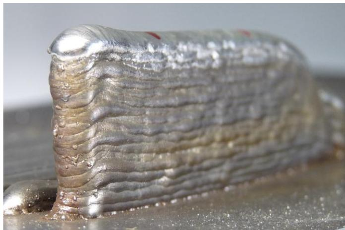
**Fig. 9:** Structure 90 x 27 x 6 mm, build by stacking single seams
