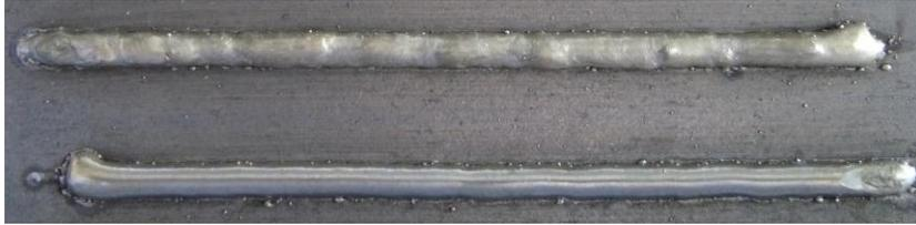
**Fig. 13:** Comparison of welding directions dragging (top) and pushing (bottom) direction
