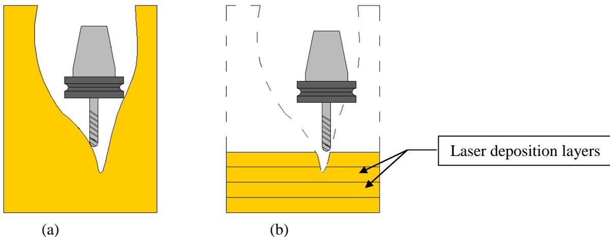
Figure (1): machining feasibility (a) machining whole part by conventional technique causes collision, (b) machining layer by layer.
