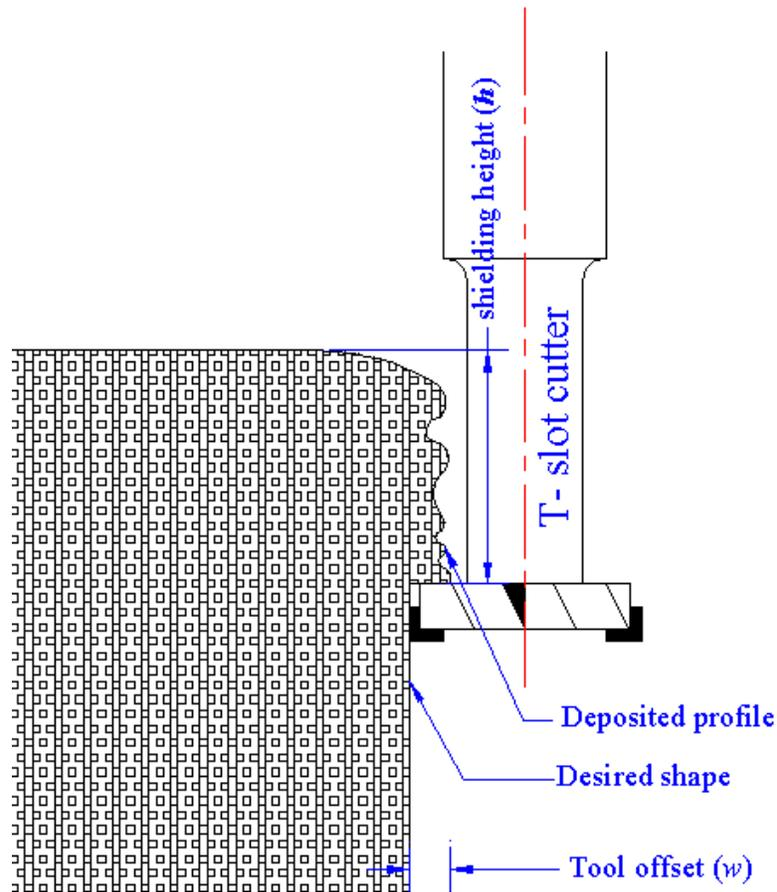
Figure (2): principle of milling machining using T-slot cutter
