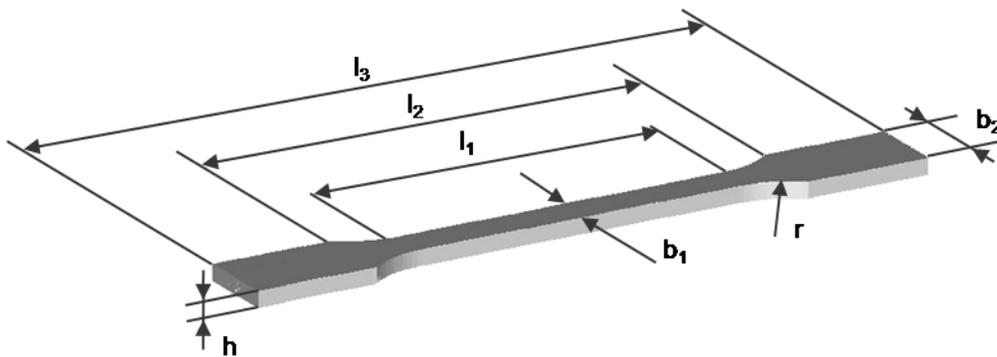
Figure 4: Tensile Testing Bar in accordance with DIN 527
