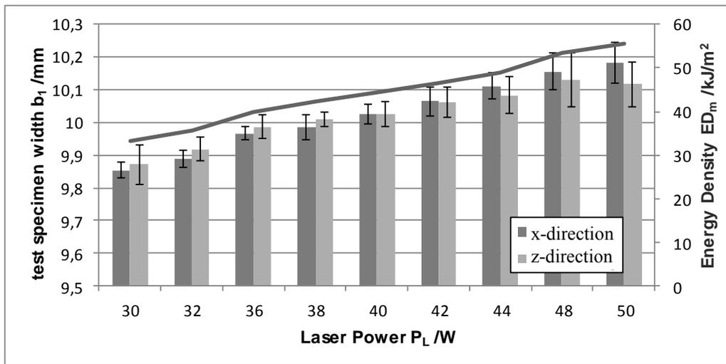
Figure 14: Measured Width of Tensile Testing Bars for different Energy Densities
