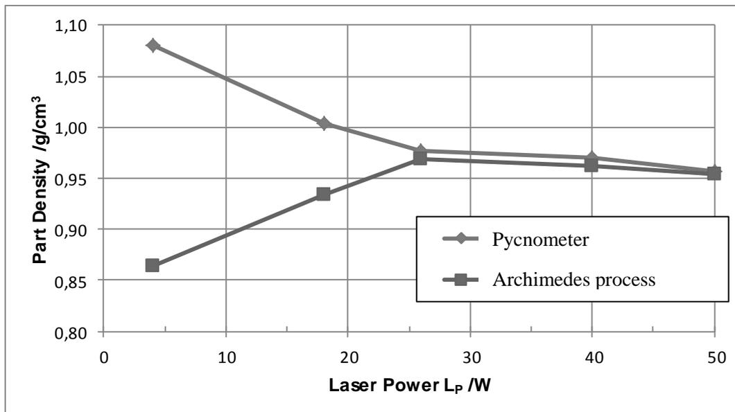
Figure 8: Comparison of the Results of the Density Measurements using the Archimedes process and the Gas Pycnometer
