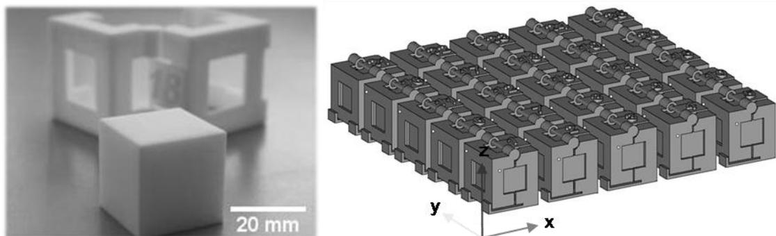
Figure 7: Test Specimens for determination of Density and creation of Thin Section Cuts
