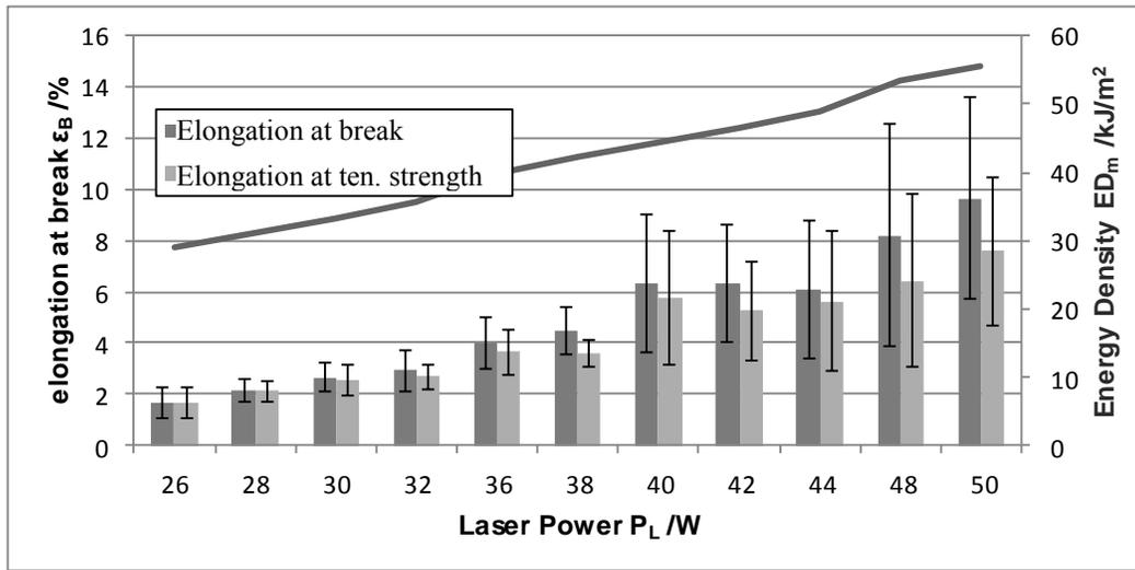
Figure 13: Elongation at break  $\epsilon_B$  for varying the Energy Density  $ED_m$  with the adjusted parameter “Laser Power  $P_L$ ”
