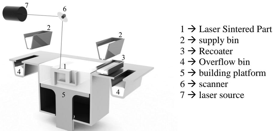
Figure 1: Laser Sintering Process [Ada10]
