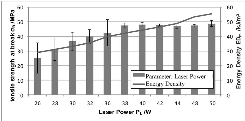
Figure 12: Tensile strength at break  $\sigma_B$  for varying the Energy Density  $ED_m$  with the adjusted parameter “Laser Power  $P_L$ ”
