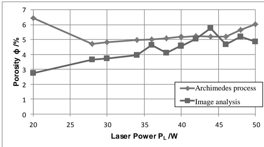
Figure 9: Comparison of the Determination of the Porosity of the Immersion Method and the Image Analysis
