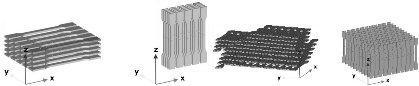
Figure 5: Arrangement of the Tensile testing Bars in a 5x5 Matrix and 11x11 Matrix
