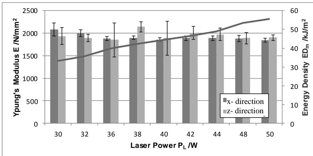
Figure 11: Modulus of Elasticity for different Energy Densities and Different Orientations
