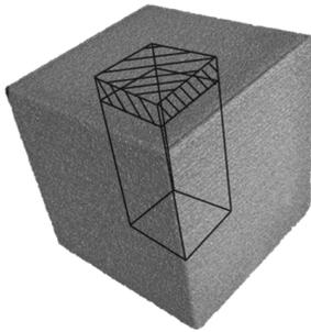
Figure 6: Cuboid to create thin section cuts
