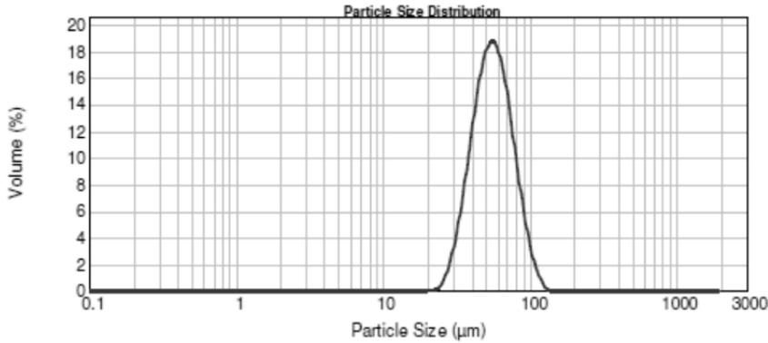
Figure 2: Volume weighted particle size distribution measured by laser diffraction
