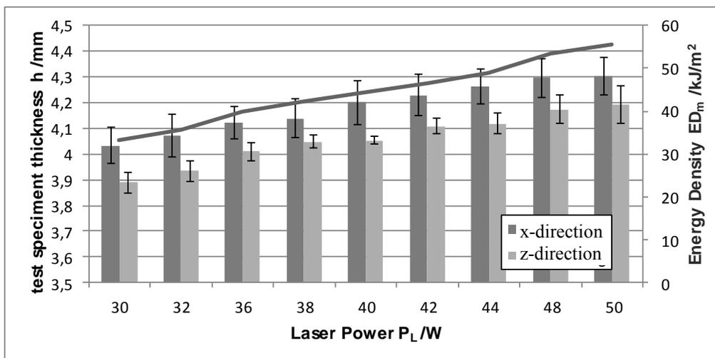
Figure 15: Measured Thickness of Tensile Testing Bars for different Energy Densities
