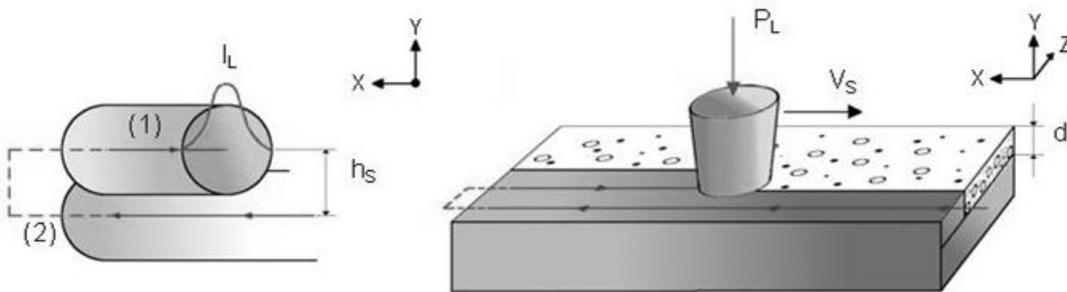
Figure 3: Schematic description for the exposure process. Left: exposure vector (1), Skywriting (2), Intensity distribution  $I_L$  as a function of beam diameter, hatch distance  $h_s$ ; Right: laser power  $P_L$ , Scan velocity  $v_s$ , and layer thickness  $d$ .
