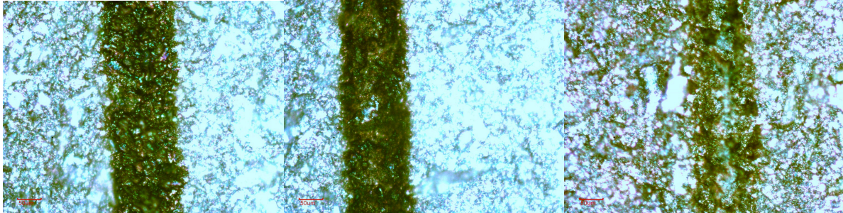
Figure 3: Single layer deposition runs of SiC on Titanium with scan speed varying from left to right, 10, 50 and 250 microns/ second. Visible light microscopy was used with a 20X objective.
