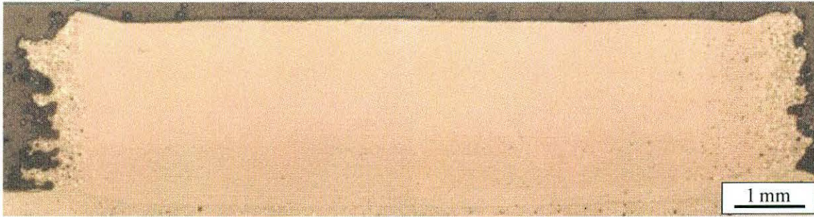
Fig. 5: Polished cross section of an alumina / zirconia compound, manufactured by SLM. Dimensions: \varnothing 18 mm x 2.5 mm 7
