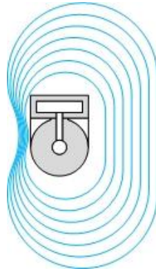
Figure 2: 2-D top-view sketch of the targeted, sized-constrained, thermal-management-structure design. The shaded regions represent a cross section through the aluminum engine's combustion chamber and exhaust manifold. The offset-concentric curves represent the targeted isotherms.
