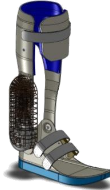
Figure 1: Conceptual model of the PPAFO showing an integrated TMS for the power source and pneumatic rotary actuator. This structure also bears mechanical loads.
