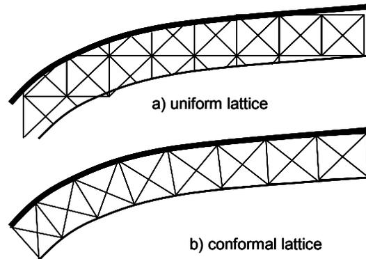
Figure 4: Uniform and conformal lattice structures
