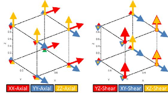
Figure 13: Loading conditions for unit-cell optimization [22]
