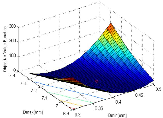
Figure 18: Design space exploration with finer resolution around the solution for the curved cantilever beam
