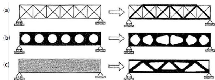
Figure 1: (a) Sizing optimization of a truss structure, (b) shape optimization, and (c) topology optimization [9]
