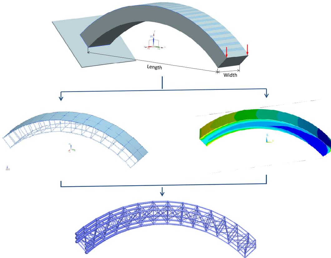
Figure 16: Final topology of curved cantilever beam using active-set method
