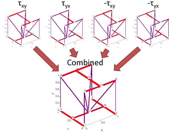
Figure 14: Combination of optimized unit-cells for shear stress in XY plane for Cantley configuration [22]
