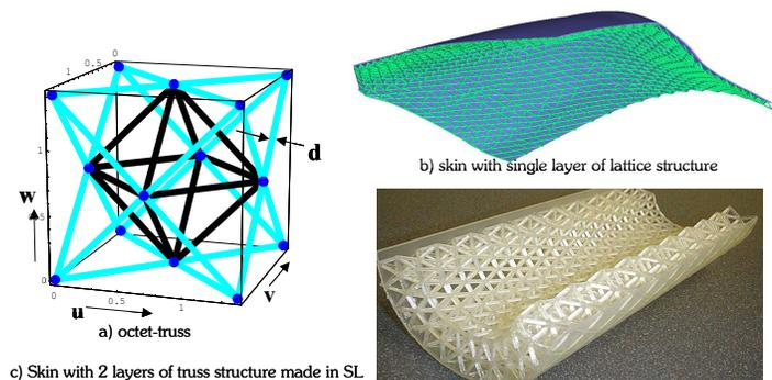
Figure 1: Octet truss unit cell and example parts with octet truss mesostructure.
