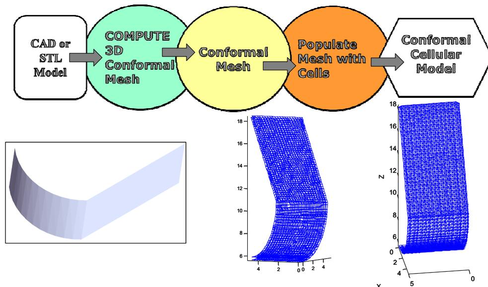
Figure 5: CLS construction method
