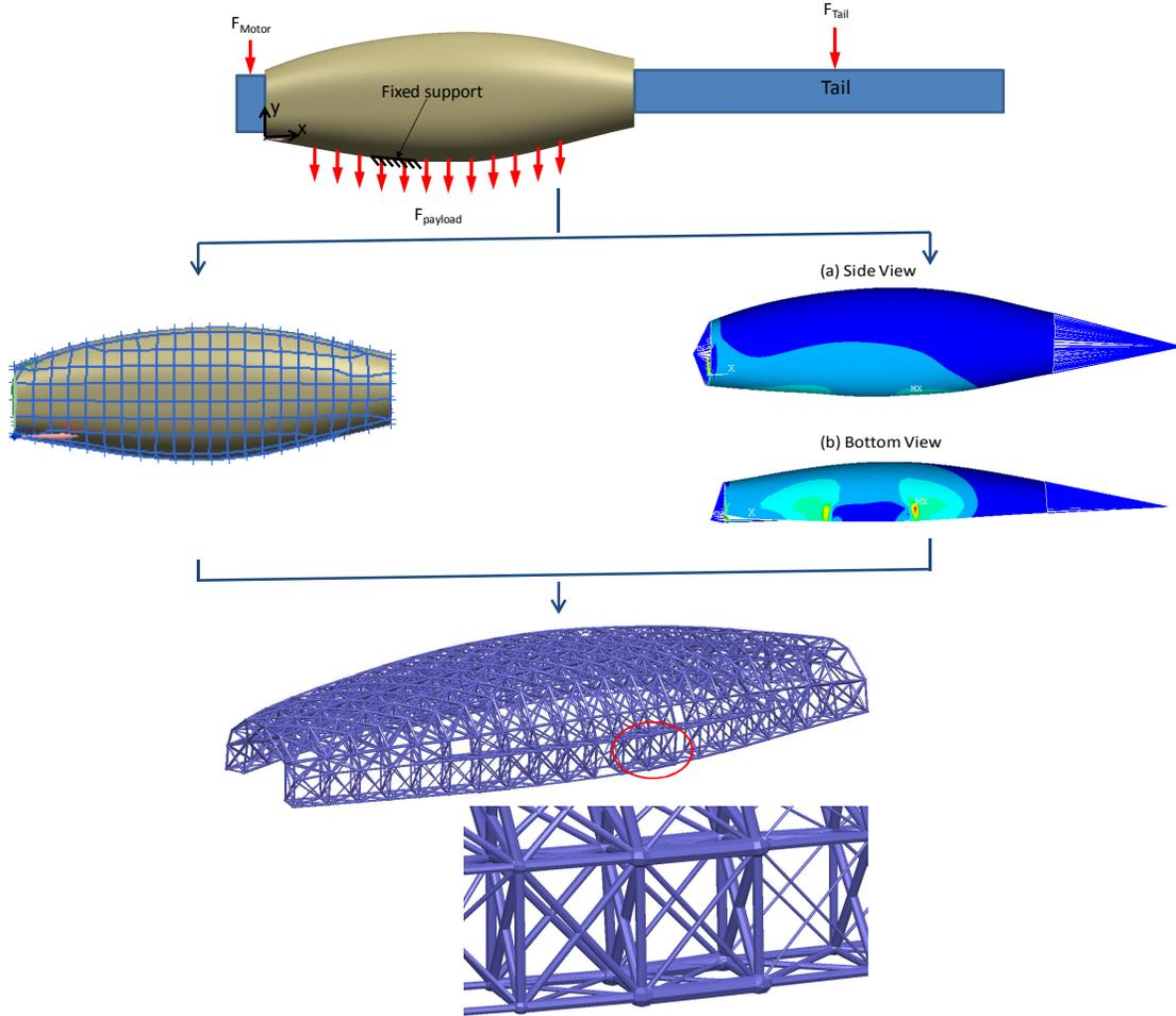
Figure 20: Final topology for the fuselage.
