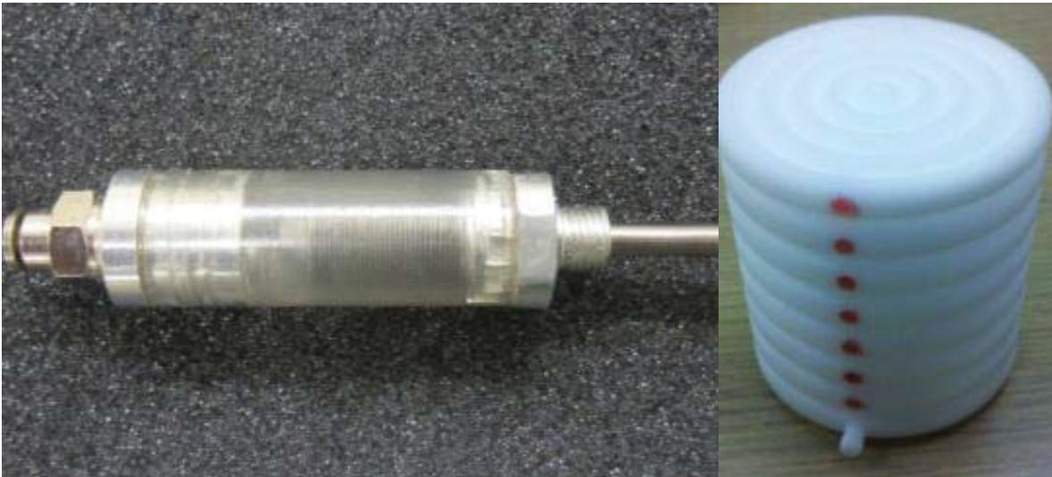
**Figure 3: Bellows actuators designed and manufactured at MSOE.**
