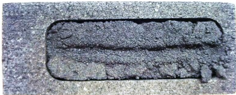
Figure 5. Plain regolith sintered at 975 °C for 1 hour
