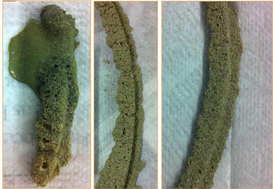
Figure 4. Extruded parts with 40%, 30% and 35% sulfur concentration (left to right)
