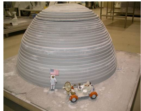
Figure 1. Top: Coextrusion by CC nozzle. Bottom: Dome structures built using Contour Crafting
