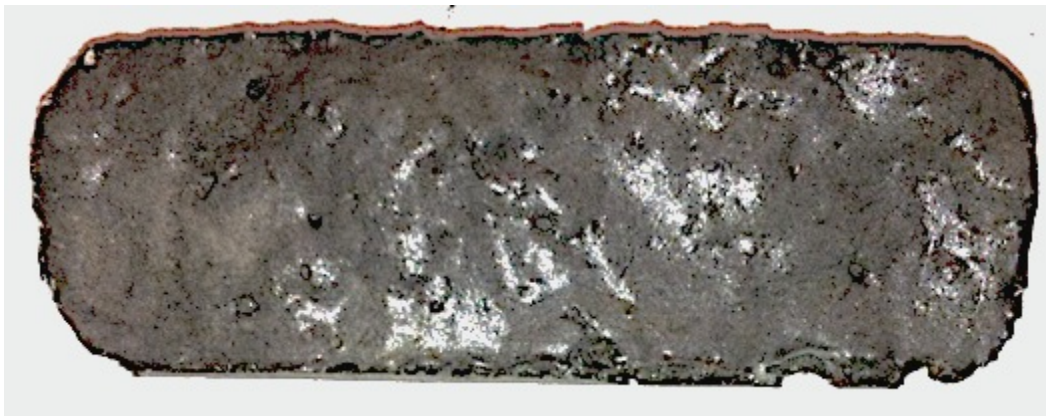
Figure 7. Plain regolith simulant sintered at 1100 °C for 1 hour
