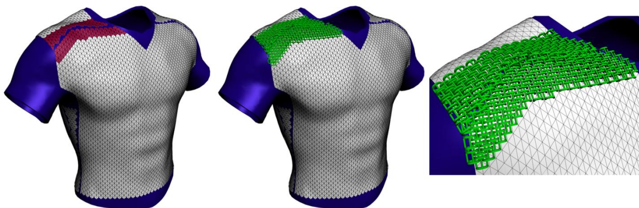
Figure 20: Seams generated between individual panels of mapped AM textile link structures
