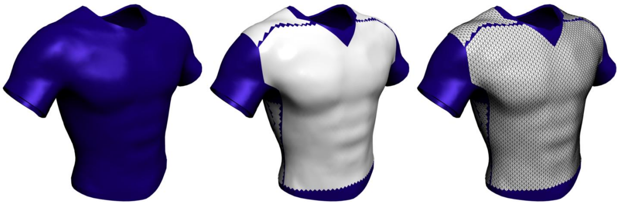
Figure 19: Target topology (left), panel layout (middle) and complete mapping mesh (right)
