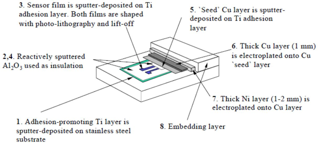
**Figure 3: Procedure for embedding thermo-mechanical thin film sensors [16]**
