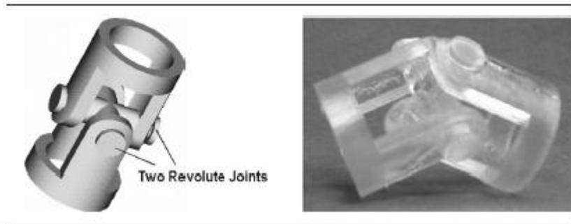
**Figure 8: Universal joint built using SL [23]**
