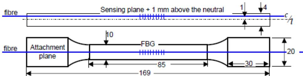
**Figure 1: Schematic of an ISO 3167 specimen with the location of the installed fiber and FBG [14]**
