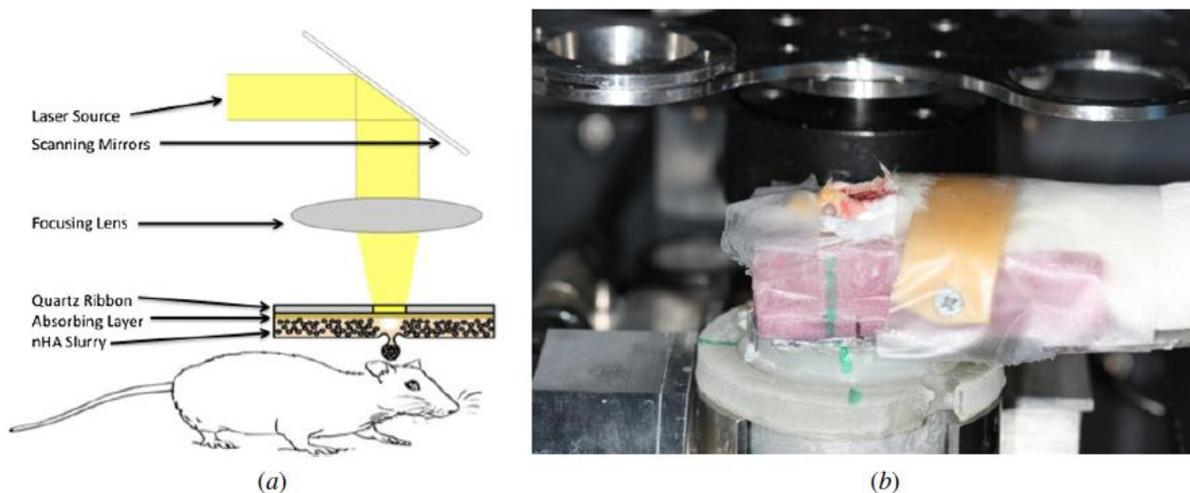
**Figure 14: a) Schematic of setup for in vivo laser printing b) Specific holder for in vivo printing in mouse calvaria defects [28]**
