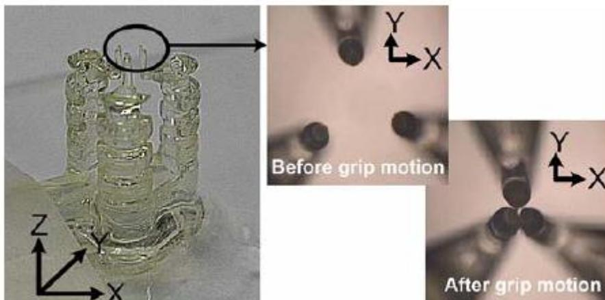
**Figure 13: Fabrication and testing of three-grip micro-gripper [25]**
