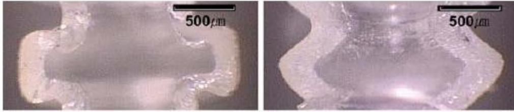
**Figure 11: Microscope images of micro bellows developed using MSL [25]**
