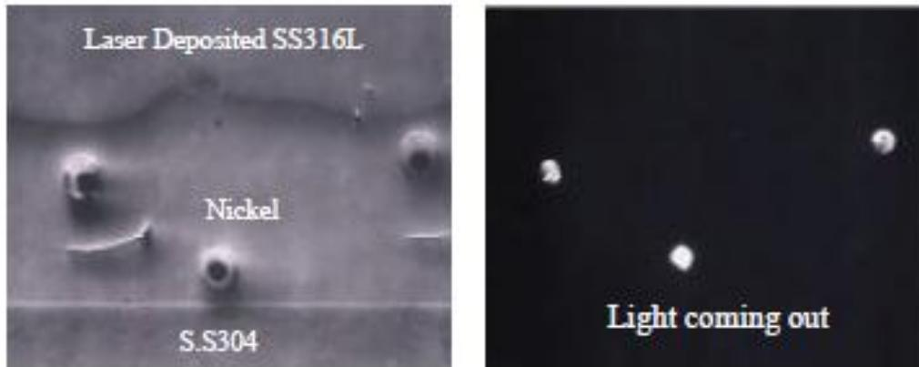
**Figure 4: Embedded fiber optic sensors [16]**
