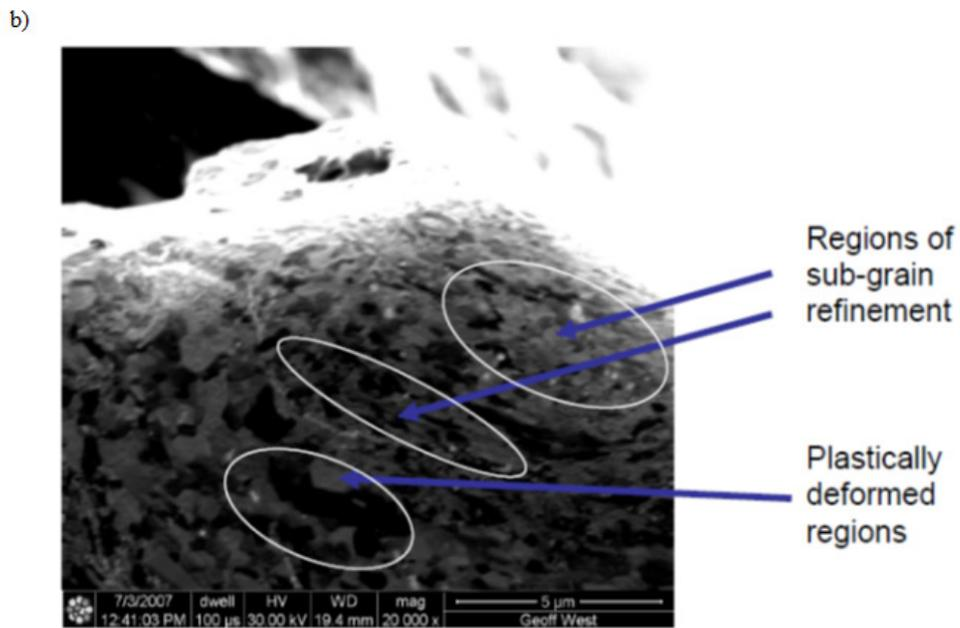
Figure 5. Ion beam induced secondary electron micrograph of (a) UC interface region showing nano-grain colonies (*i.e.* regions of dense nano-grain sized sub-grains) outlined [10] and (b) top of welded foil layer that experienced direct sonotrode contact
