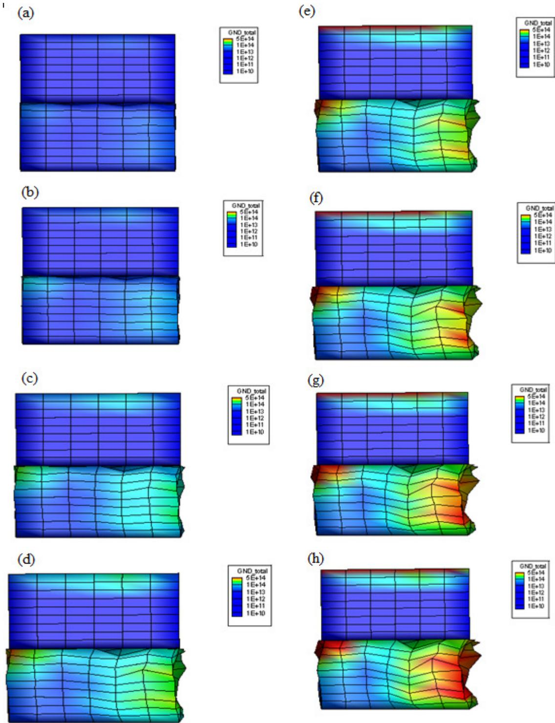
Figure 4. GND evolutions at (a) 10, (b) 20, (c) 50 ((i) onset of significant GND evolution: top surface-top foil and (ii) frictional sliding to sticking), (d) 80, (e) 100, (f) 120, (g) 140 and (h) 160 cycles. CPU time advantage attained is 2000:1.
