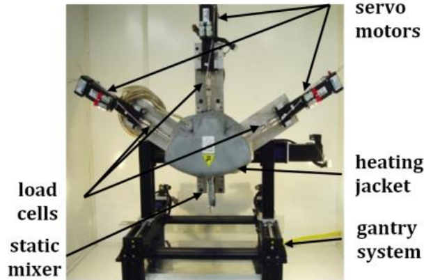
Figure 1. The triple-extruder Freeze-form Extrusion Fabrication (FEF) machine.
