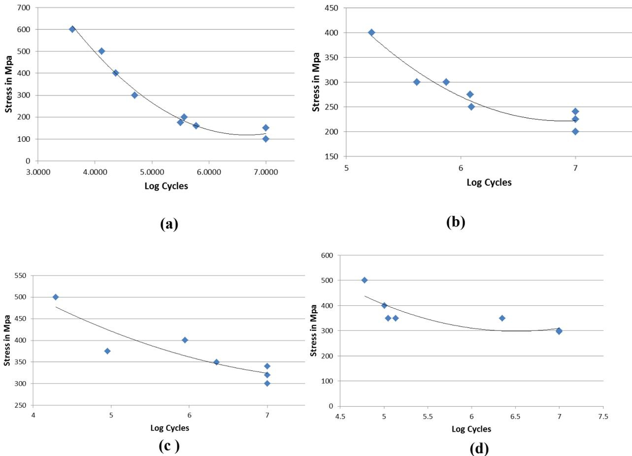
Fig.3. Stress Vs. log cycles to failure for EBM built Ti64 samples. a) Vertical as-built samples b) Horizontal as-built samples c) Vertical machined samples d) Horizontal machined samples
