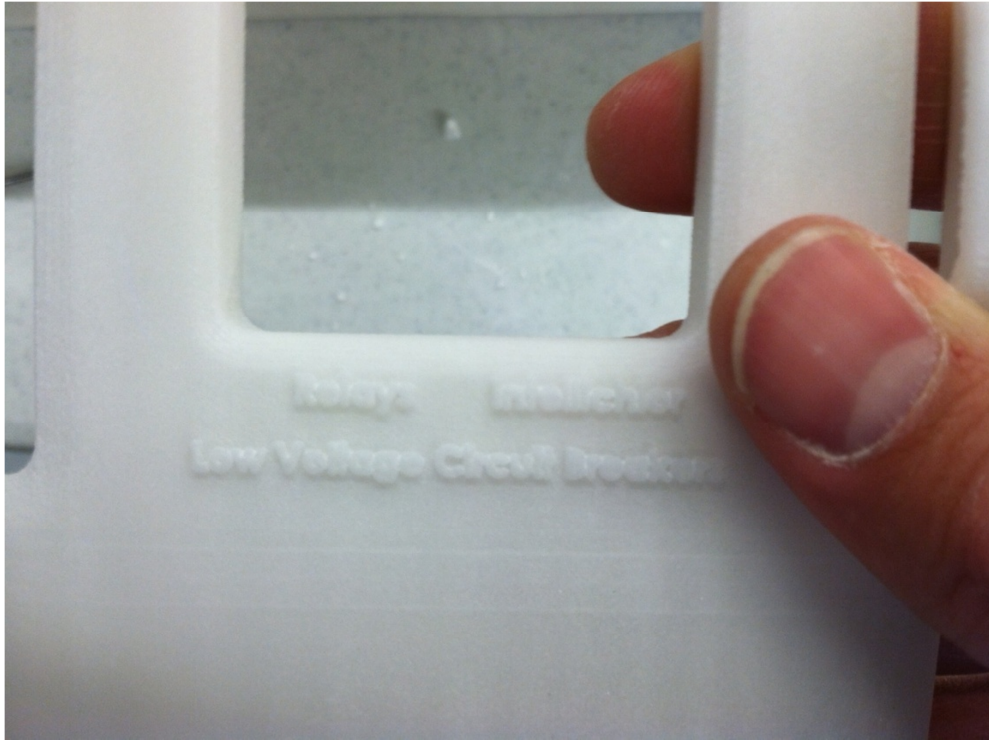
Figure 8. Feature detail using Rilsan® Invent Natural powder
