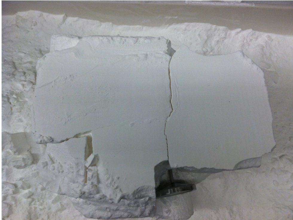
Figure 9. Part cake using Rilsan® Invent Natural powder
