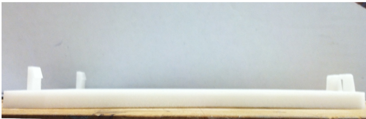
Figure 7. Prototype built with Rilsan® Invent Natural powder displaying minimal warping
