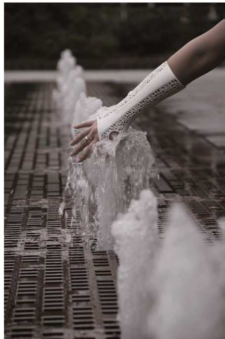
Figure 3: Bespoke-fitting wrist splint fabricated using Selective Laser Sintering (EOS P100 system and Polyamide 12/PA2200 powder). Image Courtesy of Fraunhofer IPA, Stuttgart.
