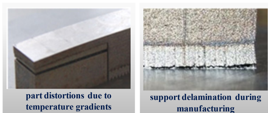
Fig. 1: Process failures of metal- and powder-based additive manufacturing
