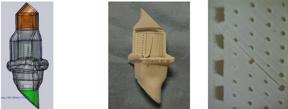
Fig 4. a. CAD model of airfoils mold b. airfoils mold built by LAMP c. cracked trailing edge
