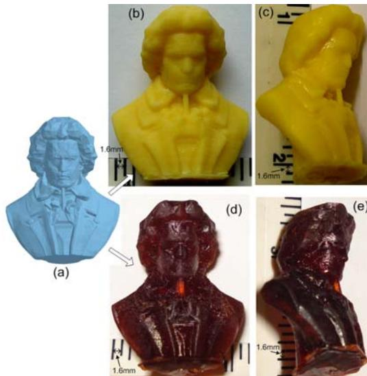
**Figure 15: A test of a statue: (a) CAD model; (b-e) two views of the built objects in two resins.**
