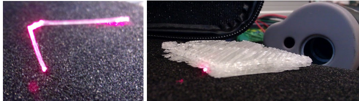
Figure 8: Optical Fibers Produced with Fused Deposition Modeling
