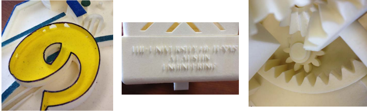
Figure 1. Examples of defects in SLS parts. L to R: unresolved walls, unreadable text, slipping gears
