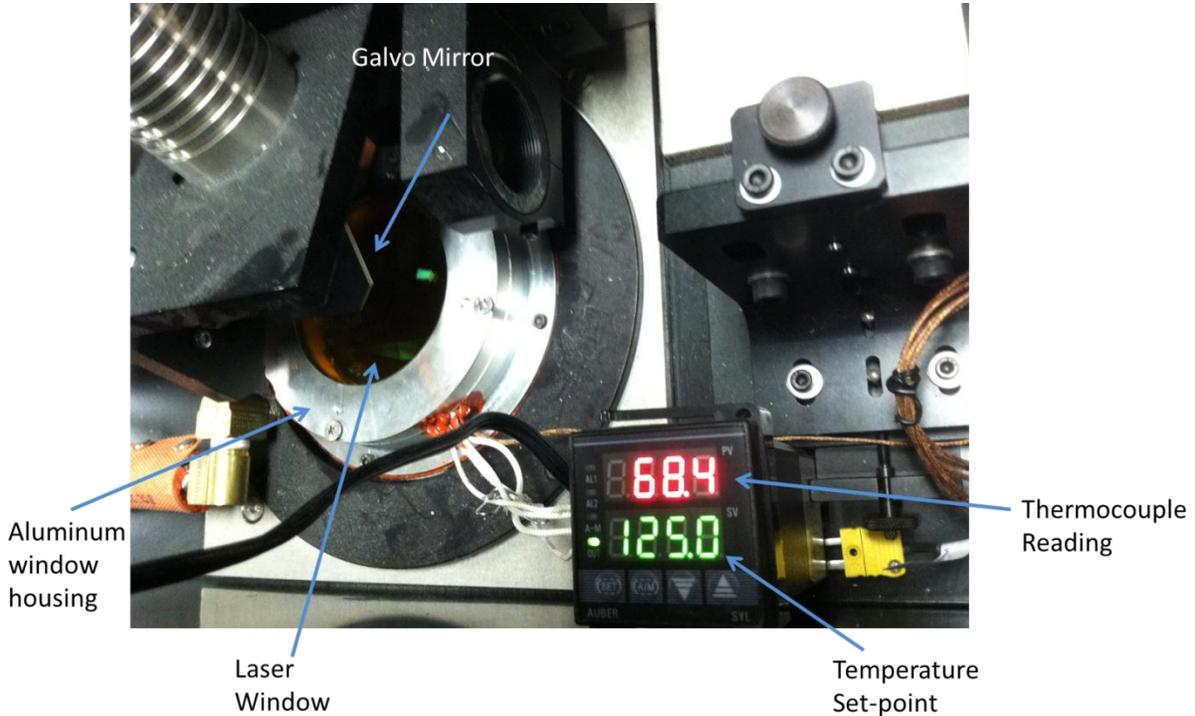
**Figure 9.** *Aluminum prototype mounted in LS machine and undergoing heating*
