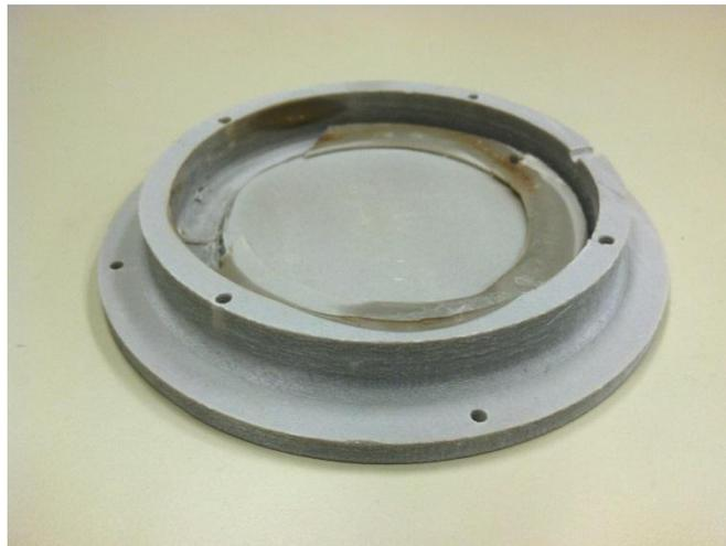
**Figure 7.** *First prototype of glass-filled PA 12 with melt-down*
