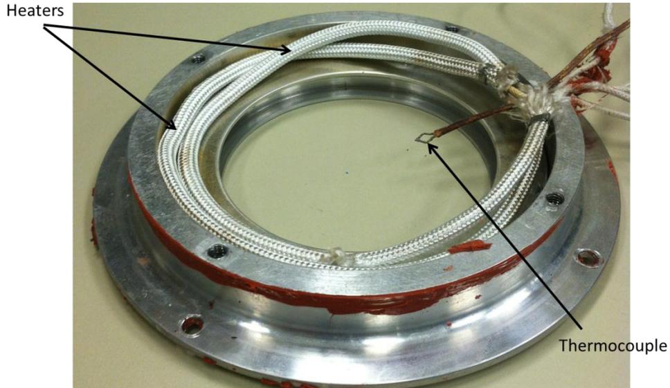
**Figure 8.** *Aluminum prototype with heaters and thermocouple*
