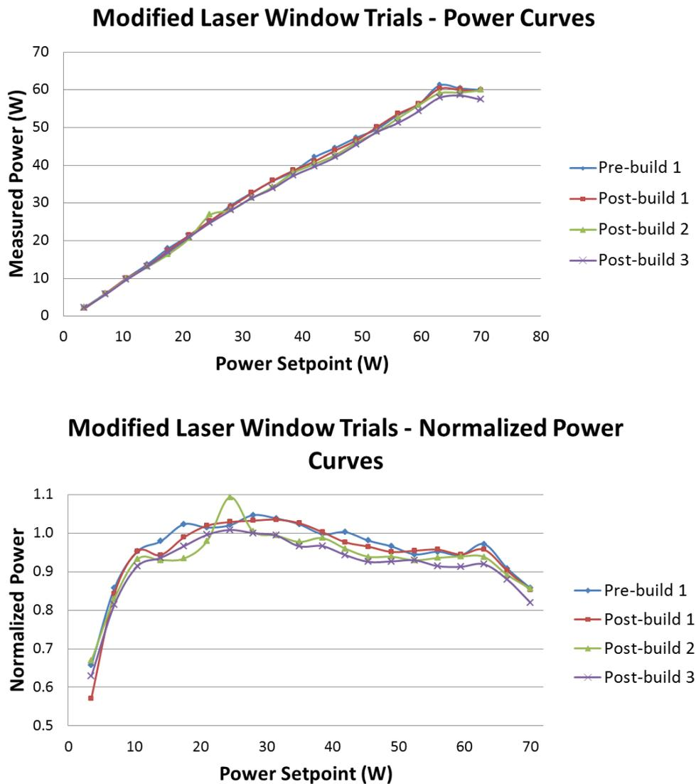
**Figure 10.** Nominal and normalized power curves for the modified window housing design
