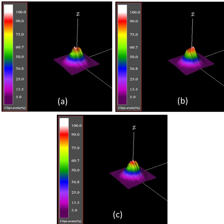
**Figure 4.** (a) 20 W, no window (b) 20 W, clean window (c) 20 W, window after 3<sup>rd</sup> build
