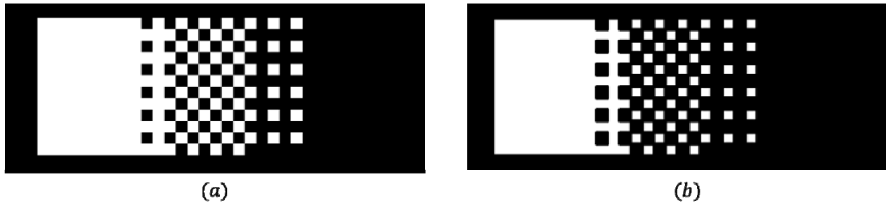
Figure 9: Erosion effect on a mask image. (a) The mask image before erosion; (b) the mask image after erosion.
