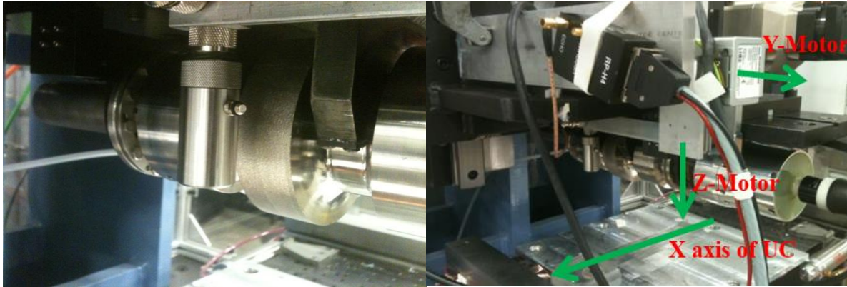
Figure 6 shows the transducer mounted on the left and the X, Y and Z axes of movement
