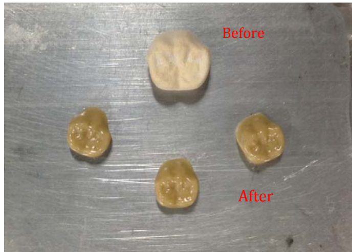
Fig. 5 Green and post sintered crown parts
