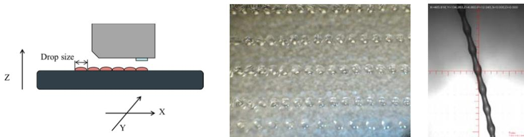
Figure 8 (a) Patterning process, (b) droplets pattern and (c) jetted fiber of pseudoplastic fluidic
