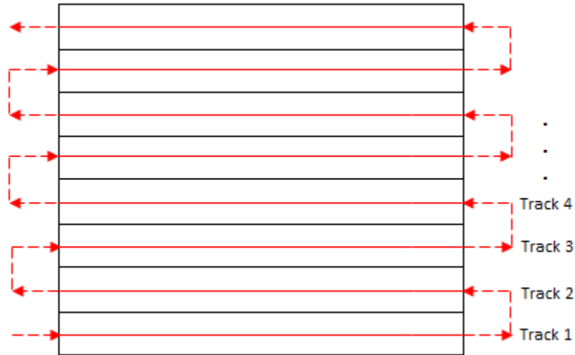
Figure 3. Scan pattern used in the model. Solid lines represent laser beam melting and dotted lines represent beam motion where a shutter blocks beam energy from reaching the powder.
