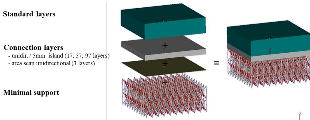
Figure 6: Sample composition for optimal number of connection layers
