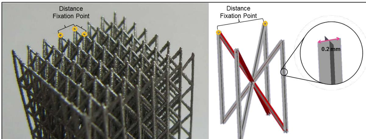
Figure 2: Realized (left) and schematic (right) of support elements
