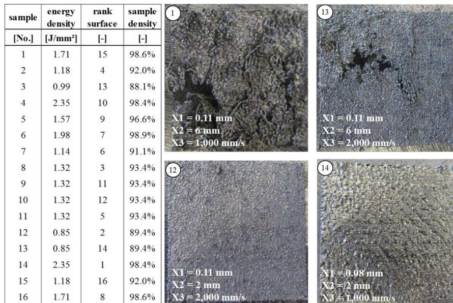
Figure 8: Resulting track energy; surface quality and density; surface examples of fine and poor results
