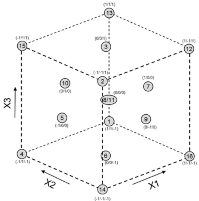
Figure 3: Graphical representation of CCD plan
