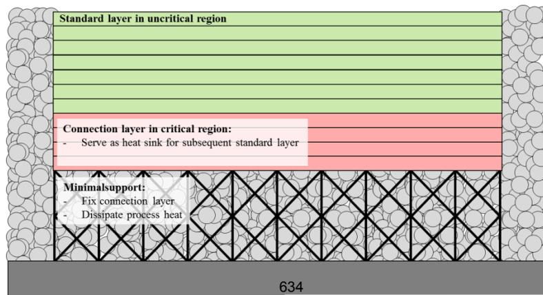
Figure 4: principle of connection layers and support structures
