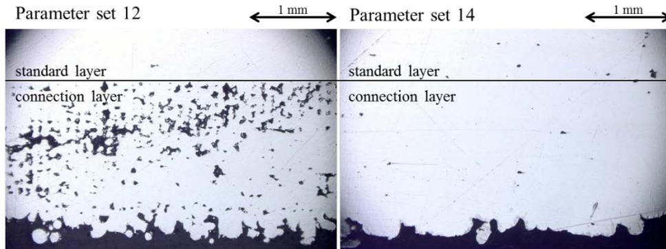
Figure 10: Polished cross section of samples 12 and 14
