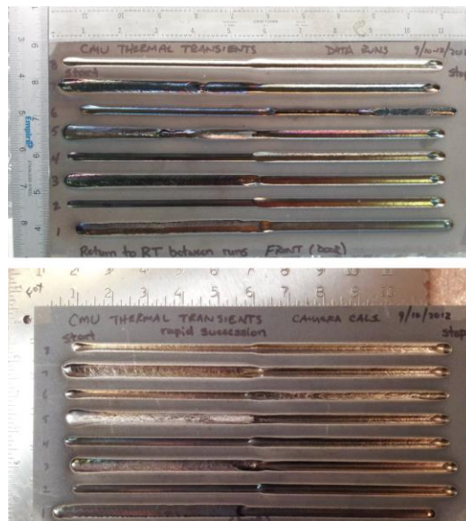
Figure 4. Experiments performed at NASA Langley Research Center. The top plate contains experiments where the plate returned to room temperature between deposition lines. On the bottom plate, depositions lines were run in rapid succession.
