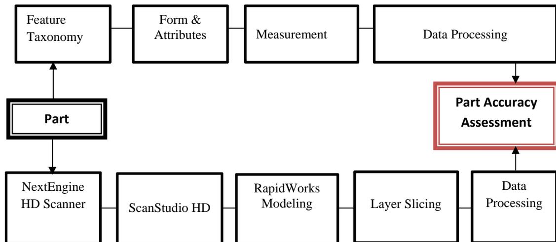
Figure 1. Hybrid method: Evaluating the accuracy of different features in a part by manual or laser scanning method
