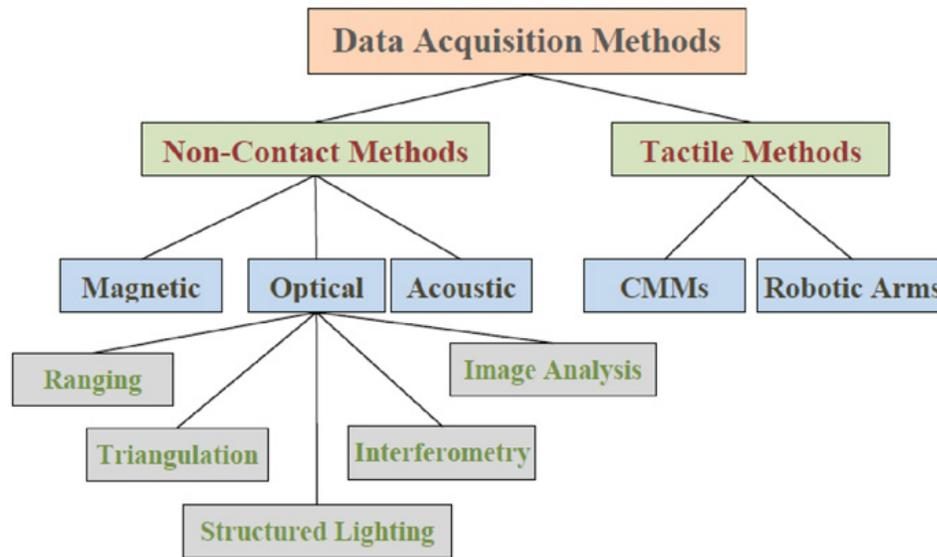
Figure 6. Data Acquisition Methods
