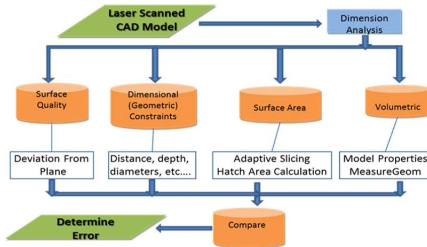
Figure 8. Four different error calculations from the digitized model
