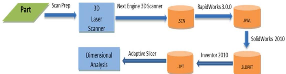
Figure 7. Data flow from physical part to digitized model
