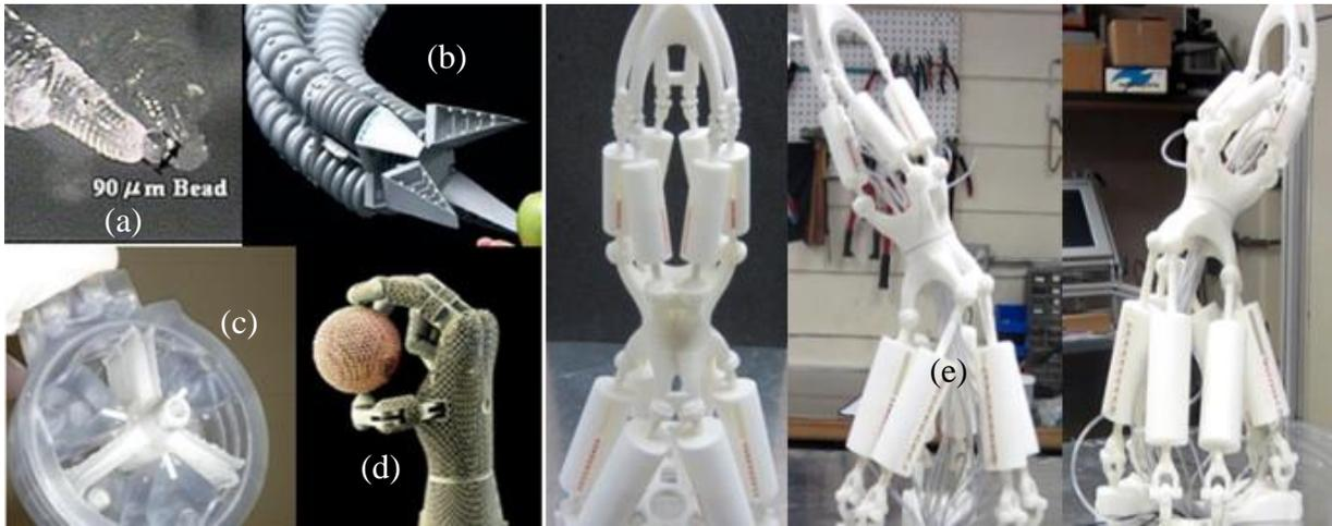
**Figure 1: Myriad of additively manufactured fluid power robots and actuators: a) SLA micro-gripper b) Bionic Handling Assistant c) MSOE's SLA rotary actuator d) Oak Ridge's titanium mesh hydraulic arm e) MSOE's simultaneously manufactured multi-level parallel manipulator.**
