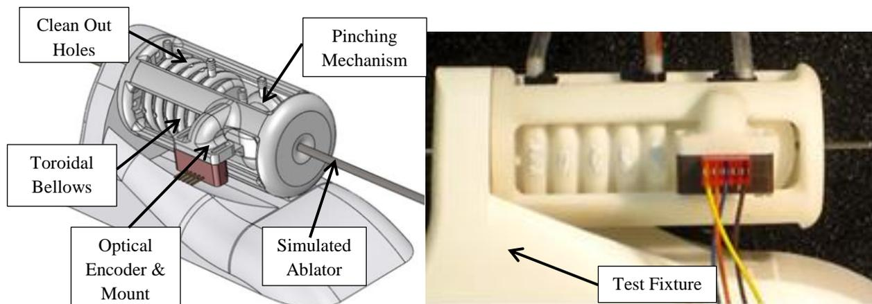
**Figure 6: MRI-compatible linear stepper motor for needle insertion.**
