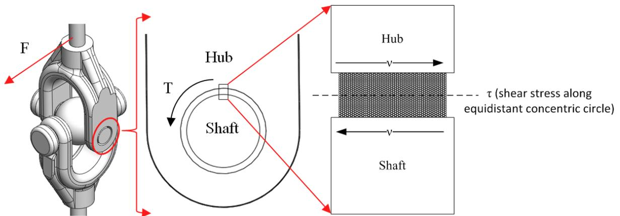
**Figure 2: Embedded universal joint depicting required force to shear unsintered powder.**
