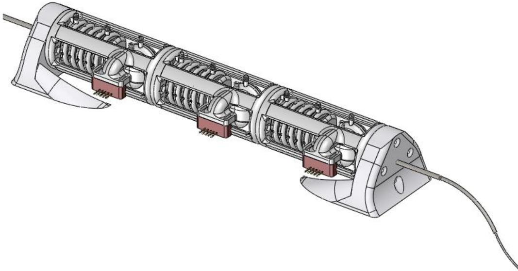
**Figure 12: Conceptual modular 5 DOF cannula robot.**
