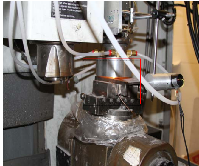
Fig. 7. Laser deposition process in progress
