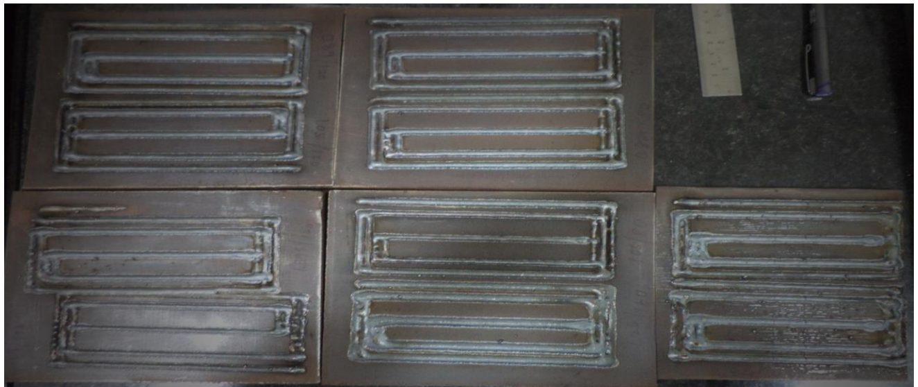
Figure 5: Weld patterns with different current and torch speeds
