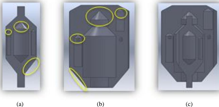
Figure 3 –CAD file (a) rotor (b) stator (c) full drawing, showing cavities with “roofs”, highlighted in yellow are 45 degree features eliminating the use of sacrificial material
