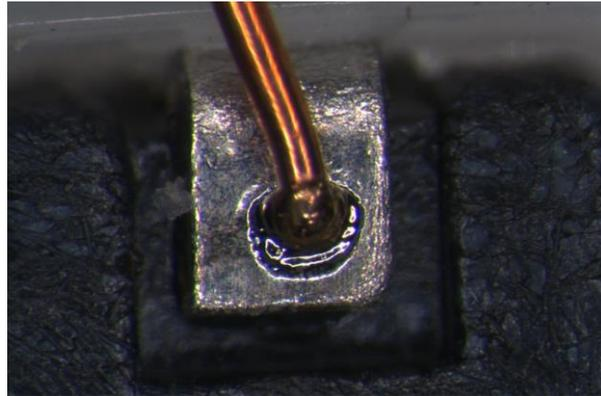
Figure 6 – Micro-Welding with YAG laser
