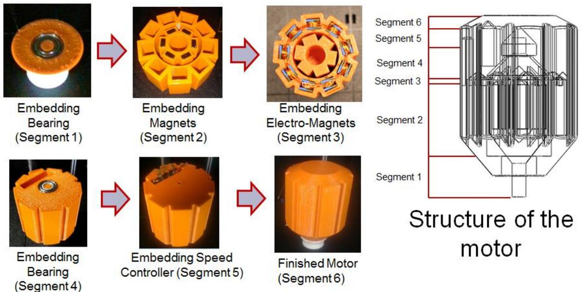
Figure 4 - Pauses in between the build
