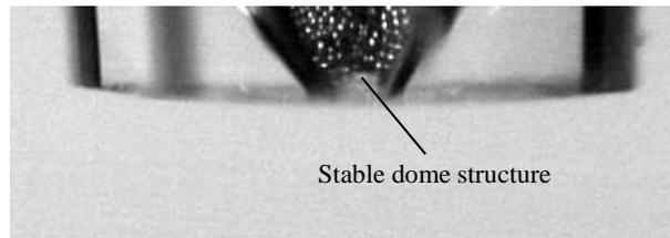
Figure 3 Dome structure of a fine powder inside the glass nozzle.
