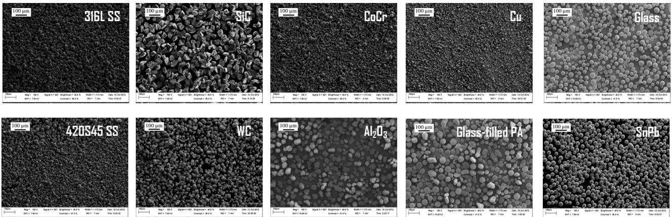
Figure 1 Scanning Electron Micrographs of the experimental powders.
