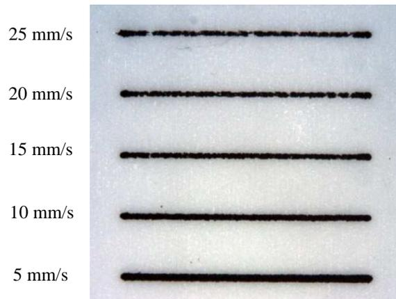
Figure 12 Printing results for copper powder obtained from different moving speeds. The nozzle diameter is 250  $\mu\text{m}$ , the signal voltage is 2 Volts and the standoff distant is 200  $\mu\text{m}$ .
