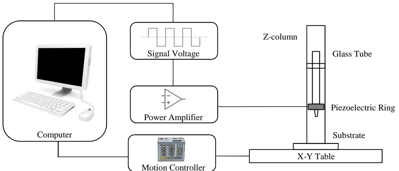
Figure 2 Schematic diagram of the dry powder printing system.
