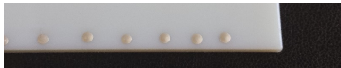
Figure 6: Droplets produced by 0.25 second dispensing pulses on VeroWhitePlus substrate
