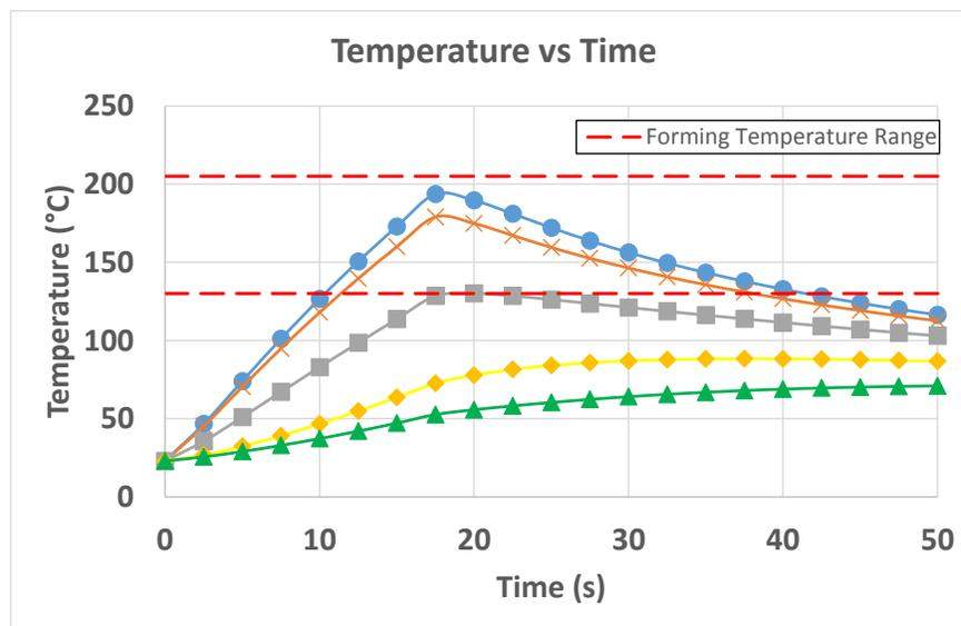
Figure 5 shows the FEA node locations and temperature profile for a joint heated on the top and bottom side by radiation for 17.5 seconds then allowed to cool at room temperature. Only the joints are exposed to the infrared radiation while a copper coating on the structure of the component reflects away unwanted radiation.
