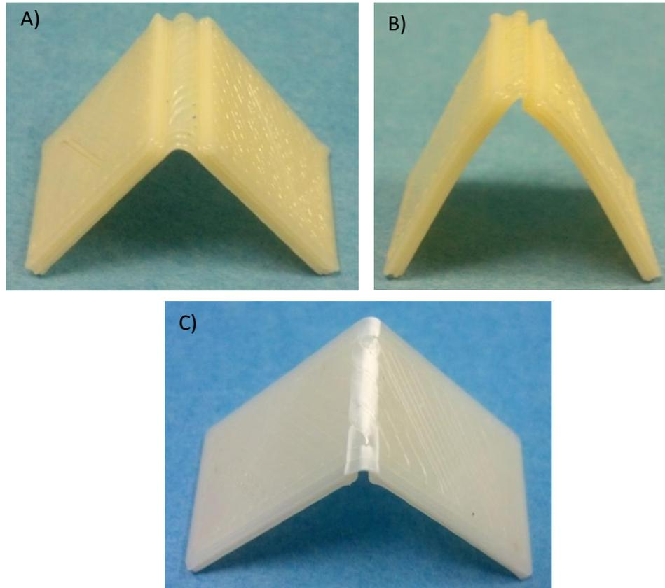
**Figure 4 A) Joint formed inside of the thermal processing range exhibits a smooth 90° bend in joint section, B) Joint formed above the thermal processing range shows signs of discoloration with warped joint and structural sections, C) Joint formed below the thermal processing range exhibits internal cracking (white area).**
