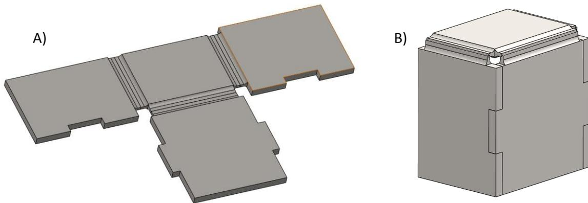
**Figure 8 Friction interface angle lock. A) Before deformation B) After deformation.**
