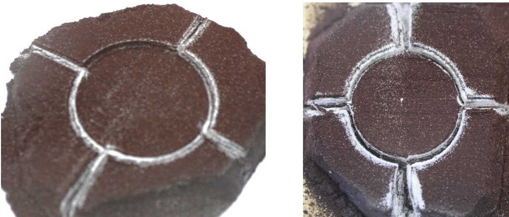
Figure 5 Sintered Ceramic Parts and Separation from the redundant material
