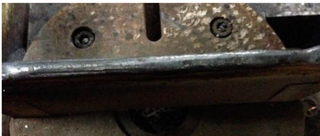
Fig.11. Surface configurations of half freeform and half rolled beads in the case the distance of vertical rolls is 6mm.
