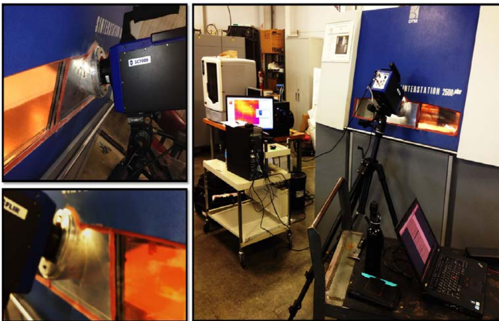
Figure 4. System setup consists of LS machine, thermal camera and a computer.
