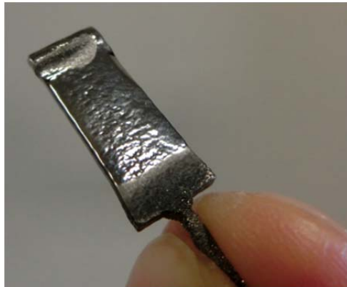
Fig.8 Electropolished sample with extraordinary surface finish
