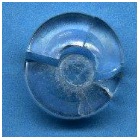
Figure 2. Extreme case of optics damage during high power laser processing.
