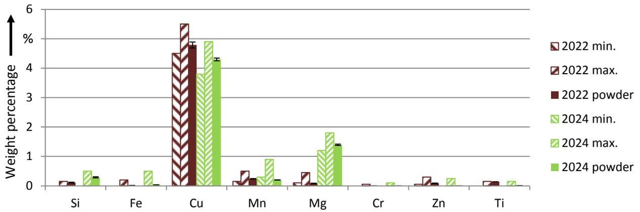
Fig. 11 Content of chemical elements in the used powders compared to upper and lower limit of respective alloy standard
