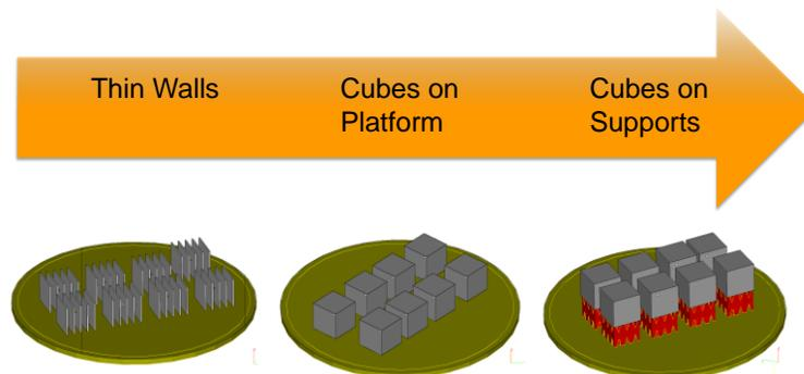
Fig. 2 The gradual approach used to assess a material's suitability for LBM
