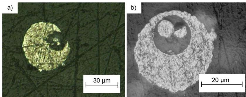
Fig. 4 Metallographical microsections of powders a) AW-2022, b) AW-2024
