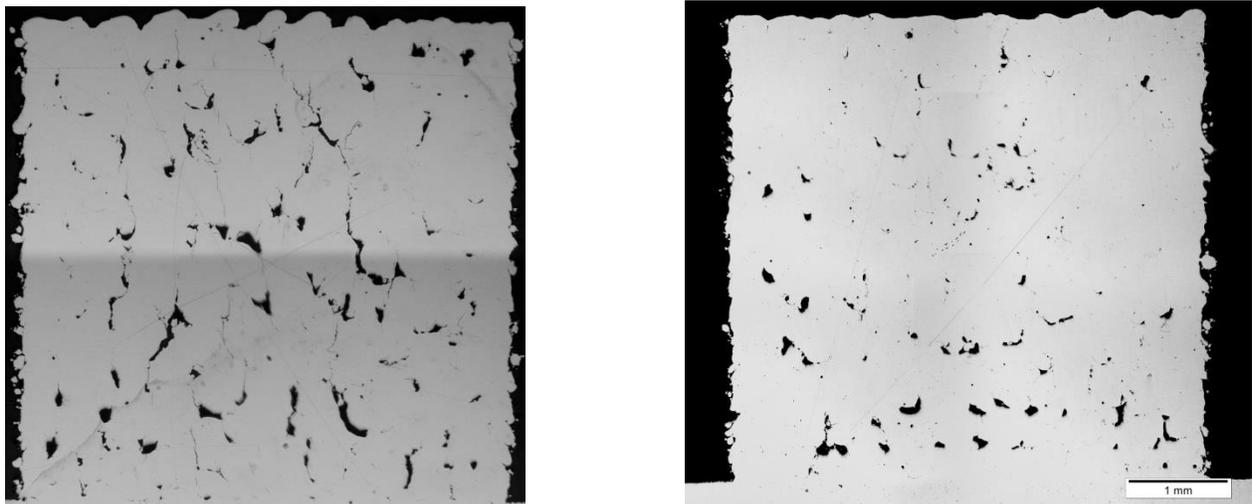
Fig. 7 Cubes on platform, left AW-2022,  $\rho_{rel} = 97.3\%$ , 100 W, 167.4 mm/s,  $d_{hatch} = 110\ \mu m$ ; right AW-2024,  $\rho_{rel} = 98.3\%$ , 100 W, 245.7 mm/s,  $d_{hatch} = 100\ \mu m$
