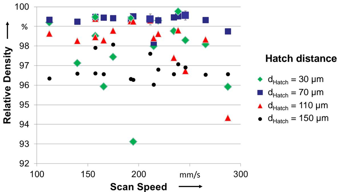
Fig. 8 AW-2022 cubes on supports, relative density over scan speed. Values including standard deviations were obtained from 3 microsections of each cube
