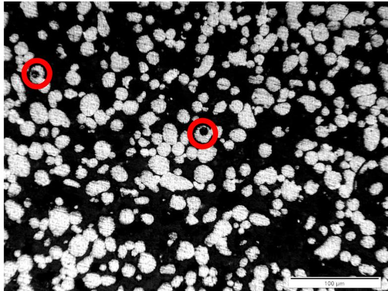
Fig. 5 Reflected-light microscope picture of microsection of powder AC-43000, highlighted in red circles: porous particles
