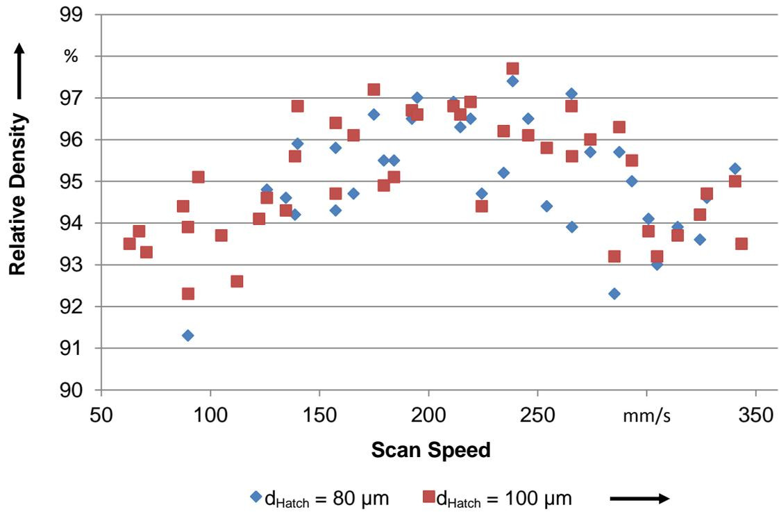
Fig. 6 Relative density of AW-2022 cubes on platform over scan speed
