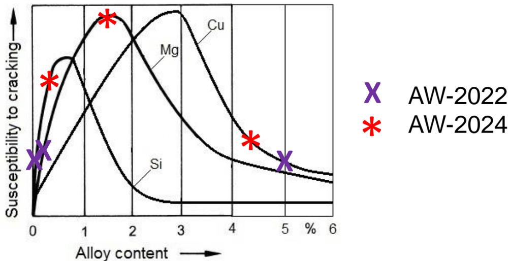
Fig. 1 Weld crack susceptibility of aluminium alloys depending on Silicon, Copper and Magnesium contents. Contents of AW-2022 and AW-2024 highlighted [16]
