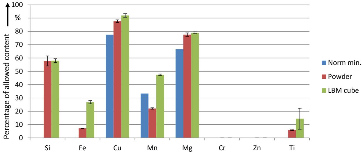
Fig. 12 AW-2024: content of chemical elements in percent of maximum value according to alloy standard, before and after Laser Beam Melting
