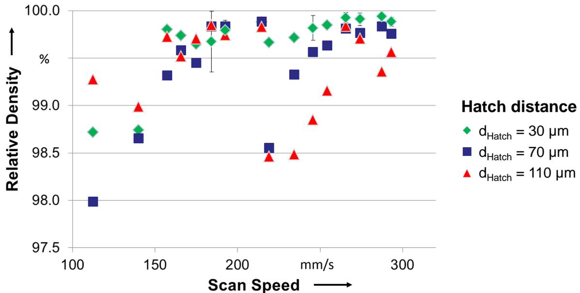
Fig. 9 AW-2024 cubes on supports, relative density over scan speed. Values including standard deviations were obtained from 3 microsections of each cube
