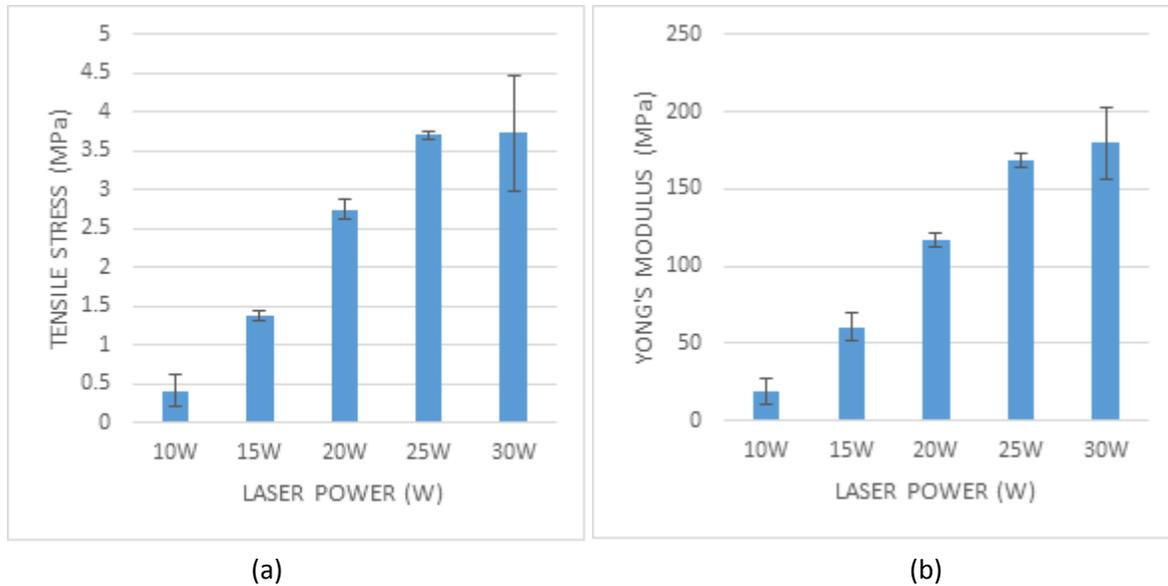
Fig. 7 Effect of laser power on (a) tensile stress and (b) Young's Modulus
