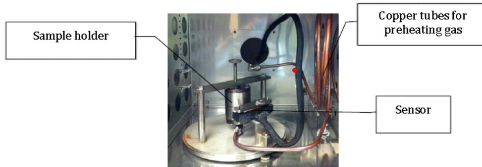
Fig. 2 Experimental apparatus for measuring the thermal conductivity
