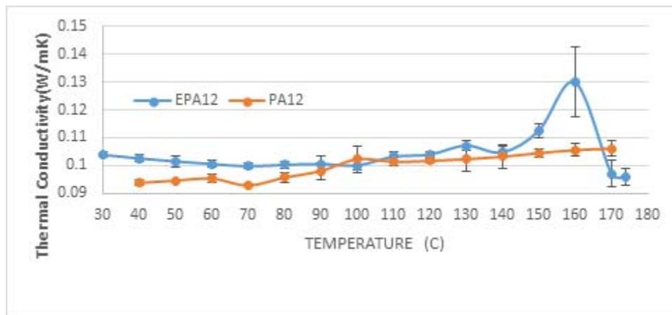
Fig. 4 Thermal conductivity of PA12 and EPA12
