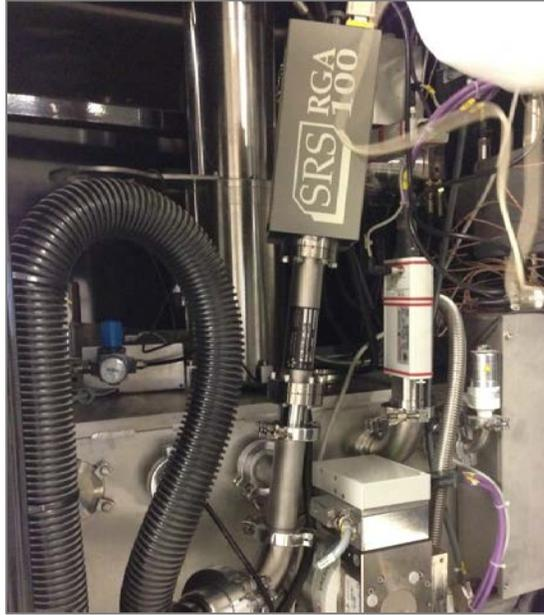
Figure 8 – RGA unit installed on the Arcam A2 system.
