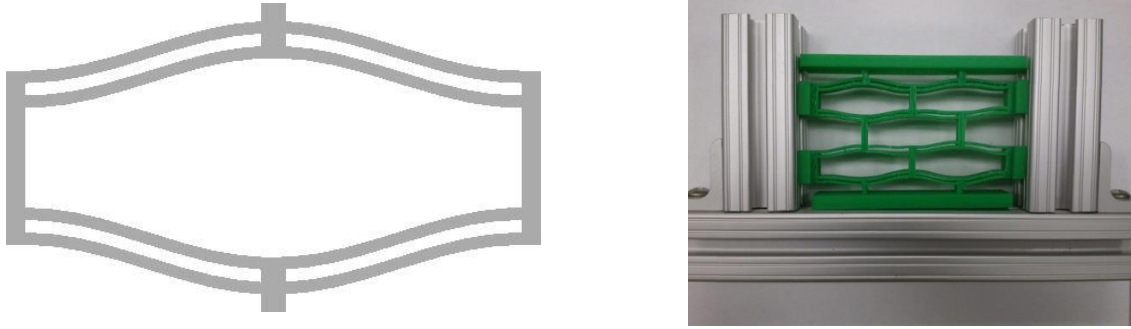
Figure 7: Primitive negative stiffness cell (left) and negative stiffness honeycomb in a supporting fixture (right).
